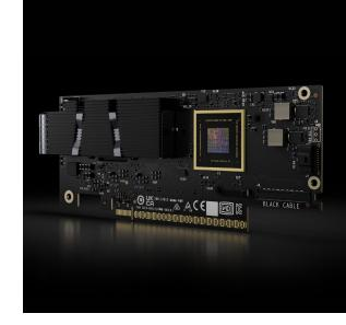
The NVIDIA® ConnectX®-8 SuperNIC™ is optimized to supercharge hyperscale AI computing workloads. With support for both InfiniBand and Ethernet networking at up to 800 gigabits per second (Gb/s), ConnectX-8 SuperNIC delivers extremely fast, efficient network connectivity, significantly enhancing system performance for AI factories and cloud data center environments.
